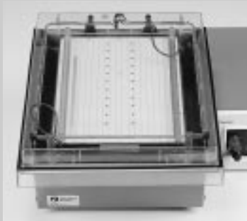
Figure 3. Multiphor II flatbed system
